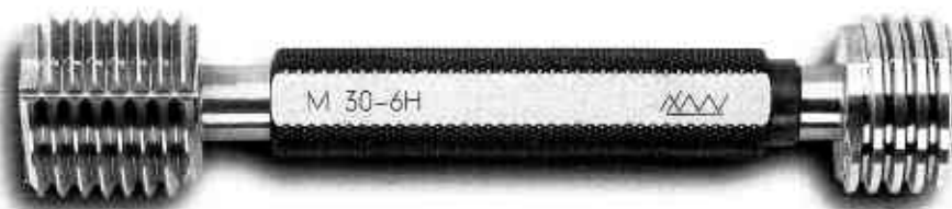
Limit thread plug gauge with piloting collar on the NO GO part and dirt groove on the GO part
